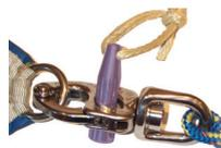
As the plug fid is pulled, the taper pries the trigger open. Great remote side release.
